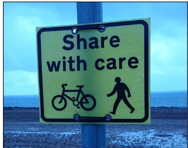
Example of a temporary 'Share with Care' sign used along the promenade to supplement standard signing to enhance the profile of the shared environment
